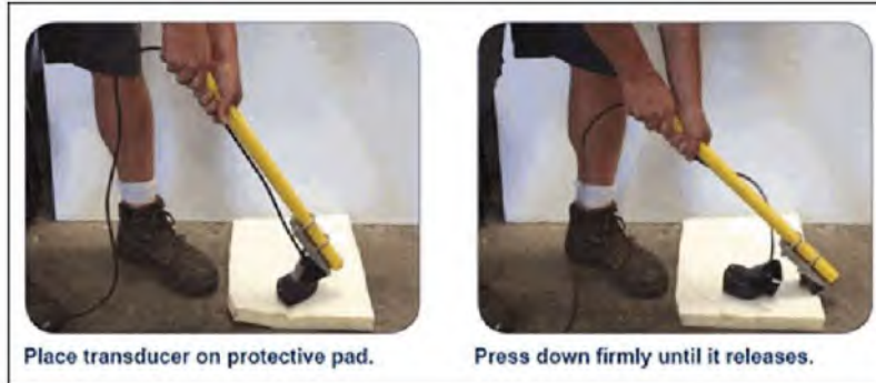
Figure 18: Removal of transducer at completion of survey.
