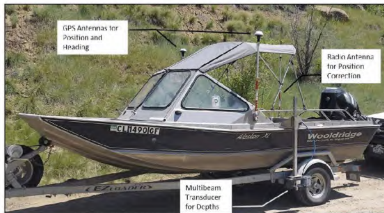
Figure 22: Multibeam bathymetry system mounted to an SRH survey vessel.
