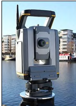
Figure 5: Backface of Trimble S7 total station should be centered over two tripod legs for efficient leveling.
