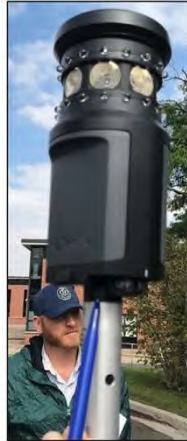
Figure 7: Robotic prism mounted on rod. End of pen is pointing to the “bottom of mount” where rod height is measured.
