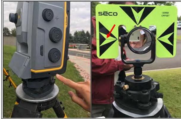
Figure 6: Bottom of black notch used to measure antennae height (left) and backsight prism black line used to measure prism height (right).
